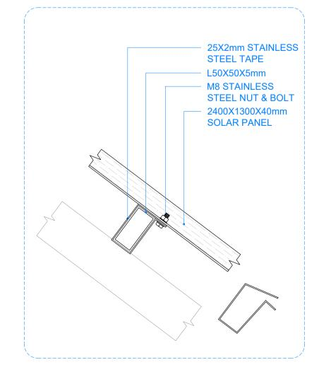
TYPICAL DETAIL OF SOLAR PANEL WITH BEAM
