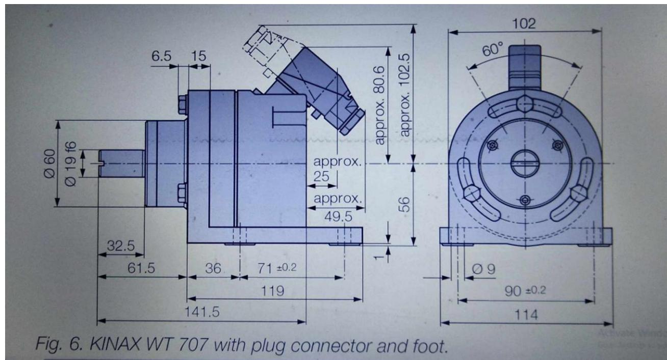
Fig. 6. KINAX WT 707 with plug connector and foot.
