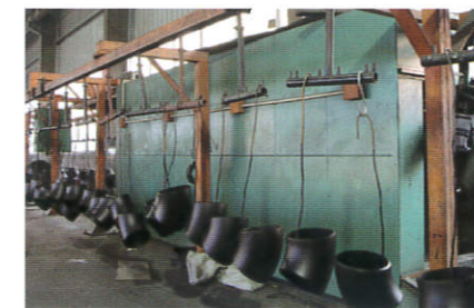
喷漆 spray paint
